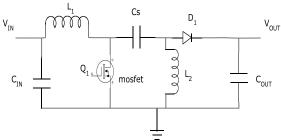
Single-ended primary inductor converter (SEPIC) is a type of DC-DC converter, that allows the voltage at its output to be more than, less than, or equal to that at its input.
