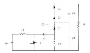
The basic difference between the normal SEPIC converter and multilevel SEPIC is the addition of diodes and capacitors. All converters have same basic operation that is the diode is opened and closed by converter operation. Basically diode is opened by reverse bias voltage this reverse bias voltage is used to charge another capacitor through diode ultimately leading to high voltage gain
